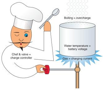
A PWM controller holds the voltage more constant. If it has two-stage regulation, it will first hold the voltage to a safe maximum for the battery to reach full charge. Then it will drop the voltage lower to sustain a "finish" or "trickle" charge. Twostage regulating is important for a system that may experience many days or weeks of excess energy (or little use of energy). It maintains a full charge but minimizes water loss and stress.
